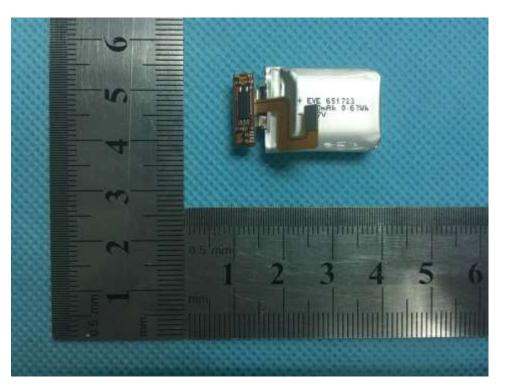
Figure 3 Inside view of battery
