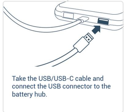
Take the USB/USB-C cable and connect the USB connector to the battery hub.
