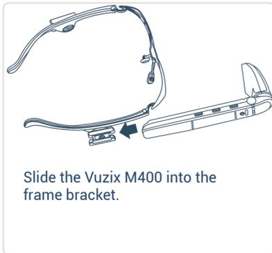
Slide the Vuzix M400 into the frame bracket.
