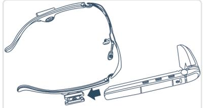
Slide the Vuzix M400 into the frame bracket.
