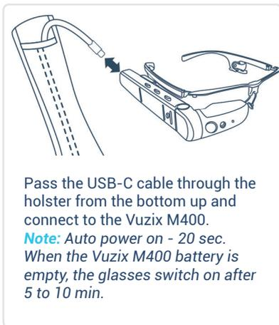
Pass the USB-C cable through the holster from the bottom up and connect to the Vuzix M400.
