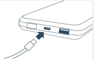
Connect the USB-C cable to the hub battery.
