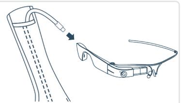
Pass the USB-C cable through the holster from the bottom up and connect to the Glass. The Glass automatically switches on.
