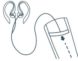
Pass the earphones through the holster, from top to the bottom.
