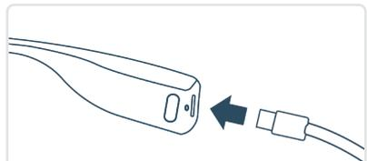
Connect the USB-C connector to the Glass. The Glass automatically switches on.
