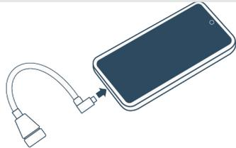
Connect the USB/USB-C (female) cable to the device.
