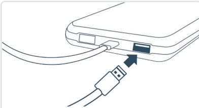
Take the USB/USB-C cable and connect the USB connector to the hub battery.
