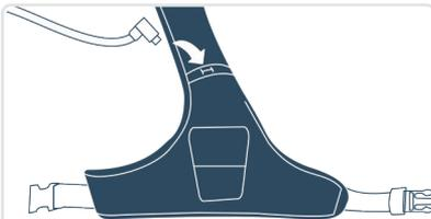
Pass the USB-C cable through the holster, from back to the front.
