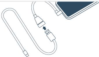
Connect the USB/USB-C (male) cable and connect it to the female connector.
